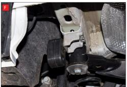
Once happy with fitment of Scorpion Exhaust, fully tighten up all clamps and fixing and plug in the electronic valve
